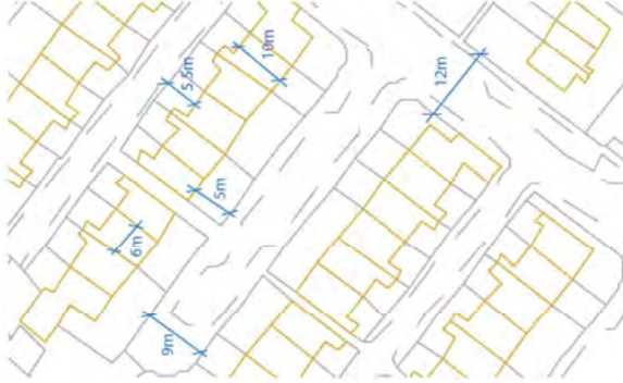
Diagram 2 Broadwalk Plot Sizes and how buildings sit on the Plot
